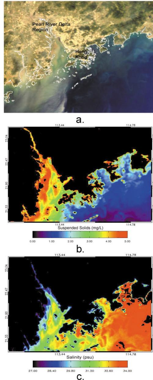
Figure 3. a. True color MODIS 500m image (Nov 03, 2003) overlaid with coastlines b. Map of suspended solids derived from multiple regression model c. Map of salinity derived from multiple regression model.
